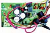
Dual Power Dual Driver Management Circuit
