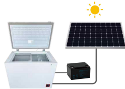
Connection1.Solar Panel + Battery + Controller + DC Freezer
